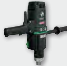
EHB 32/4.2 1.700 W; 215/330/460/680 min -1 ; Ø 32 mm in Stahl
