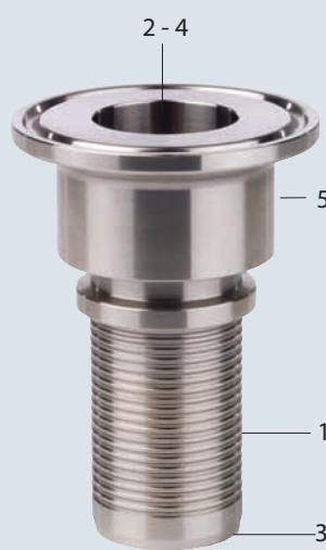
1. Lightly-grooved hose shank for assembly with EN 14420-3 RK safety clamps, HRRK or HRP-swage ferrules
