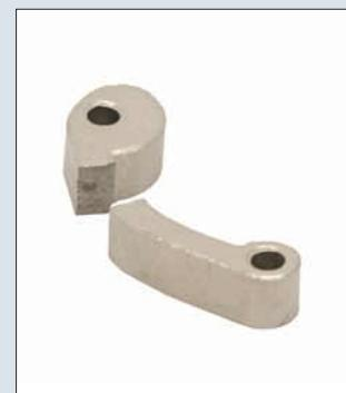
Fractured sintered handle
