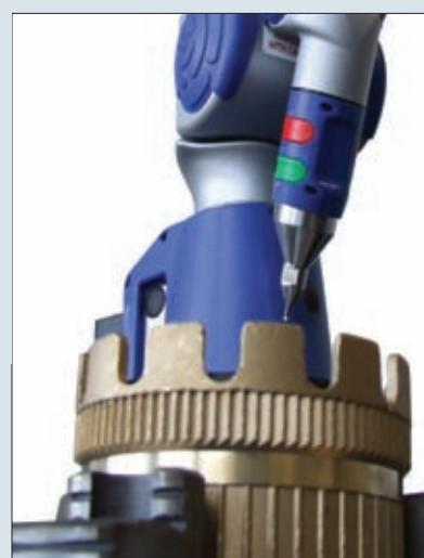
Using the gauges required by the European EN 14420-6 standard, LMC-Couplings measures the following four quality-point dimensions of its TW couplings:
